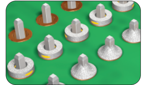
Bare pins, washers in place pre-reflow, post-reflow
